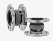
Suitable transfer of up to 100% hydrogen as well as for 100% methane or other mixtures ('Hythane'). Due to their low permeation, they can be used for any kind of piping systems in the industrial sector and for ships. operating pressure 25 bar (2,5 MPa).
