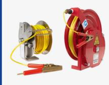
Reel with spring rewind mechanism. Frame available in polyester powder coated steel, UV resistant or stainless steel and any colour. High visibility grounding cable, up to 30m, DN 6mm and different types of clamps.
