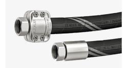
H2 hydrogen hoses for low-pressure range,  $\Omega/T$  connection hoses for the transfer up to 100% hydrogen. Continuous smooth inner lining. Robust hose construction with 20 bar (2 MPa) operating pressure with a very low permeation of < 0.36 Ncm³/h. H2 hoses DN 13-50 available with crimping ferrules, Spannloc or Spannfix clamps.
