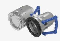
Nozzle with automatic shut-off, check valve, 1-speed lever latch with removable latch pin EB 280. Body aluminium, chemically nickel-plated and plastic-coated. Spout fiber-reinforced composite plastic with integrated misfilling protection, no dripping when removing nozzle from fill point. Inner parts stainless steel and POM, strainer PA. Lever and guard PA. Scuffguard and comfigrip PVC, seals NBR and PU. Includes EW 22 test adapter.
