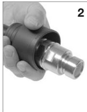
Push break sleeve **BS 19** back over the breakaway part and hose fitting.
