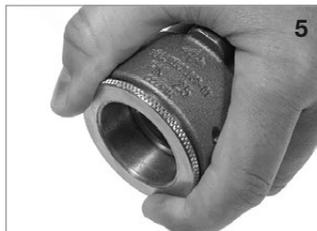
Push back the sliding sleeve of the body and hold it.
