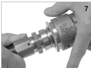
Release the sliding sleeve – it remains in its position. Now push in firmly the breakaway part until the limit. The sliding sleeve will snap back. Check the coupling for tightness.
