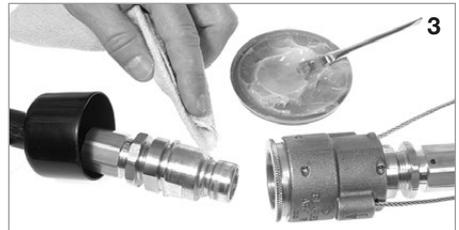
Clean all **ARK** parts and check them for damages like damaged sealing surface of the breakaway part, deformations, broken plastic parts or damaged lanyard. With such damage the coupling must be exchanged. Except for the visible O-ring EO 146 LT no spare parts are supplied. The body and breakaway part shall not be separately replaced or substituted.
