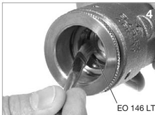
Slightly lubricate the O-ring within the body.
