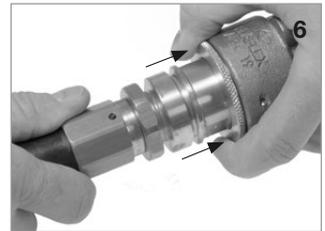
Fit the breakaway part into the body.
